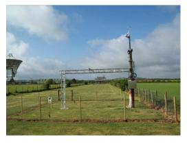
The measurements produced by the sonic anemometer/gas analyser system (aside from gas concentrations and wind velocity resolved into 3 orthogonal components) are friction velocity, vertical water vapour and carbon dioxide fluxes and sensible and latent heat flux.
