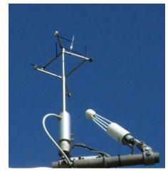
lower troposphere that makes the technique possible. In order to properly measure the turbulent properties of the atmosphere the measurements must be made at a high frequency - 20 Hz for the Chilbolton Observatory system.
