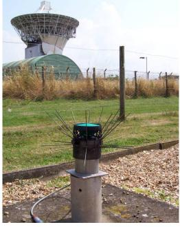
The system provides an instant response to the onset of rainfall and changes in rainfall rate and drop size distribution, without any delay such as occurs in raingauges which rely on collecting rain in a funnel. It allows a link between direct rainfall measurements and the deduction of drop size from radar reflectivity measurements using the 3 GHz CAMRa radar.
