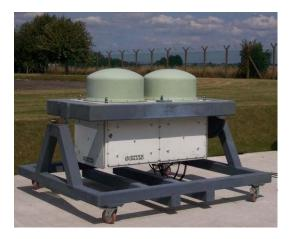
The radar provides real-time measurement and display of the full Doppler spectrum and of the spectral moments Z, v, and w. Full time-series of I and Q data may also be recorded for more detailed off-line studies.
