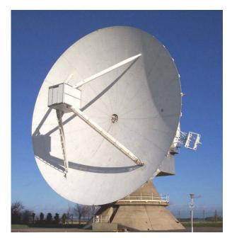
Typical research areas for which CAMRa is used include rainfall rate estimation, hydrometeor characterization (with aircraft verification), effects of precipitation on terrestrial and earth-space radio propagation, multi-wavelength studies of cloud and precipitation, clear-air and boundary-layer investigations and satellite sensor ground-truth verification. It is operated on a case-study basis.
