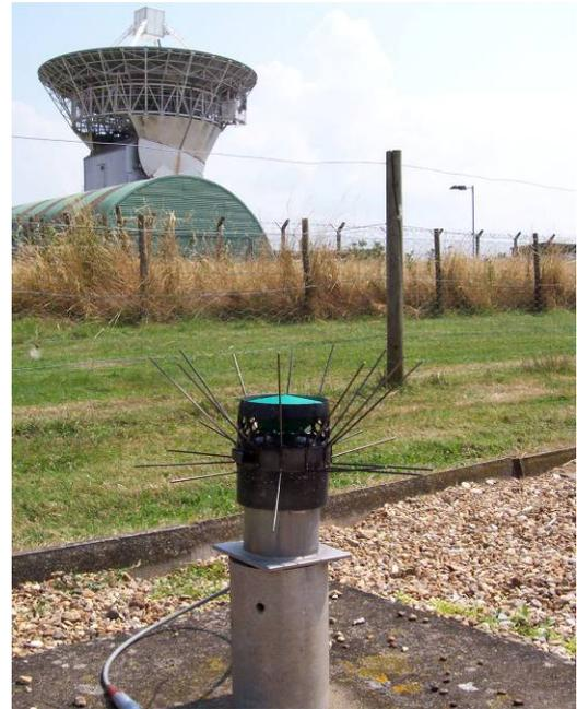
The system provides an instant response to the onset of rainfall and changes in rainfall rate and drop size distribution, without any delay such as occurs in raingauges which rely on collecting rain in a funnel. It allows a link between direct rainfall measurements and the deduction of drop size from radar reflectivity measurements using the 3 GHz CAMRa radar.
