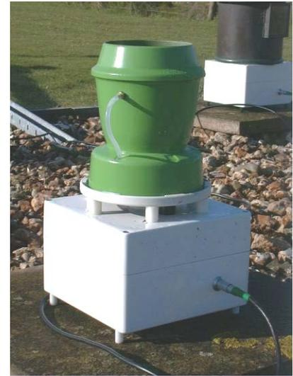
The benefit of this technique is the rapid response to rainfall. A single drop is equivalent to 0.004mm accumulation of precipitation (based on the standard collector), compared to the standard tipping bucket gauge, which triggers with 0.2mm accumulation of precipitation. Rainfall rate can be estimated by equating the volume of water recorded with the collecting area.
