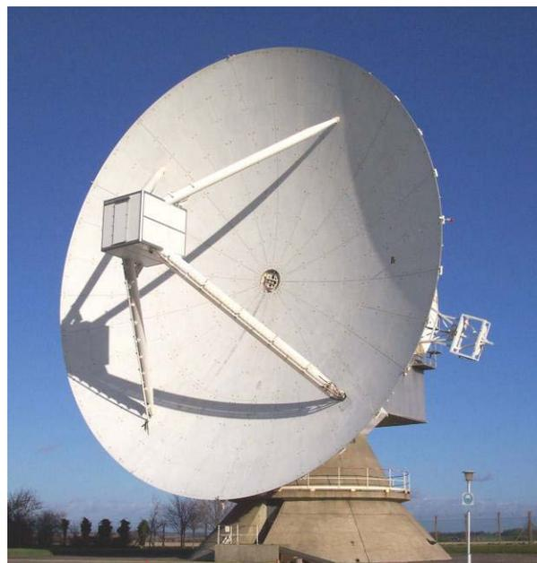
Typical research areas for which CAMRa is used include rainfall rate estimation, hydrometeor characterization (with aircraft verification), effects of precipitation on terrestrial and earth-space radio propagation, multi-wavelength studies of cloud and precipitation, clear-air and boundary-layer investigations and satellite sensor ground-truth verification. It is operated on a case-study basis.
